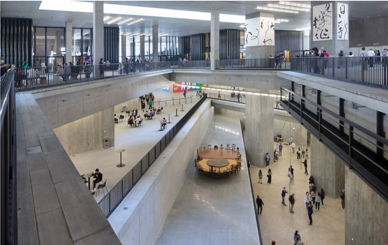
The vast openings on each floor could accelerate smoke spread, increasing the risks associated with fire incidents
