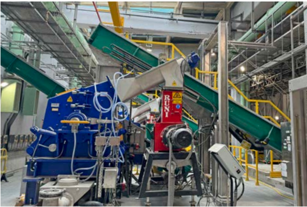
The hammer mill in O·Park2, first of its kind in Hong Kong, provides a comprehensive solution to purify and separate organics before digestion
