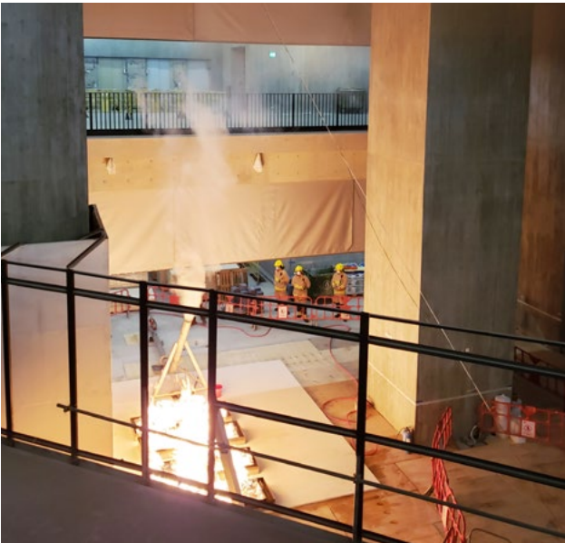
On-site long-throw sprinklers test (left) and hot smoke test (right) were conducted to provide invaluable insight into the effectiveness of fire safety strategies
